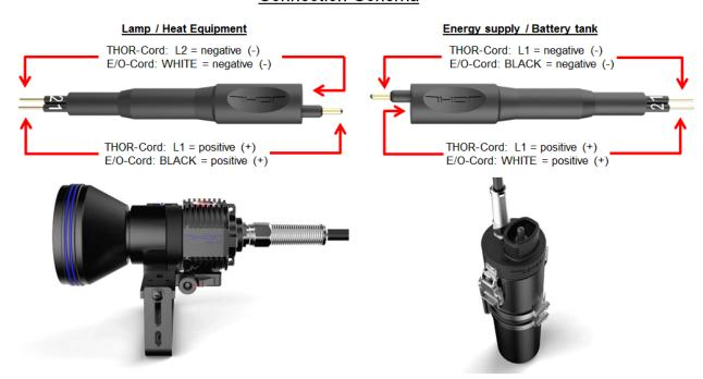
Attention! To avoid confusions or irreparable damages of the equipment by short circuits, measure the basic occupation of the Cords to be exchanged (plug & socket) and the polarity before changing!
